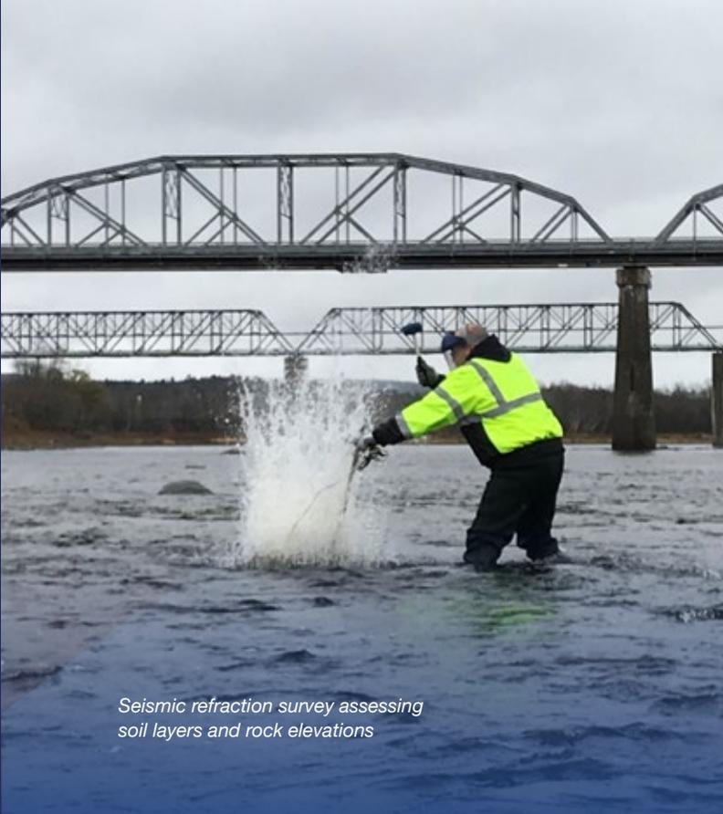
*Seismic refraction survey assessing soil layers and rock elevations*
