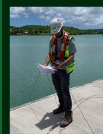
*Corrosion potential survey of a pier in St. John's, Antigua*
