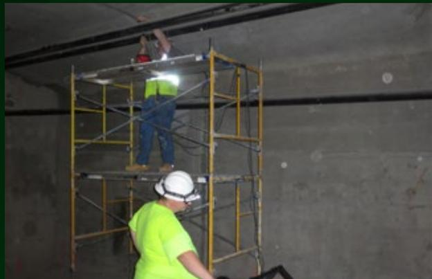
*Acoustic testing of external tendon for grout defects, Sarasota, FL*
