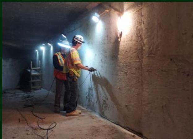
*Post-tension void detection using sonic/ultrasonic testing
