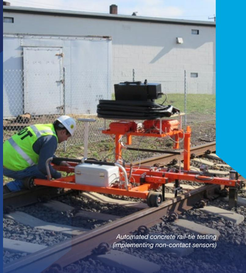
*Automated concrete rail-tie testing (implementing non-contact sensors)*
